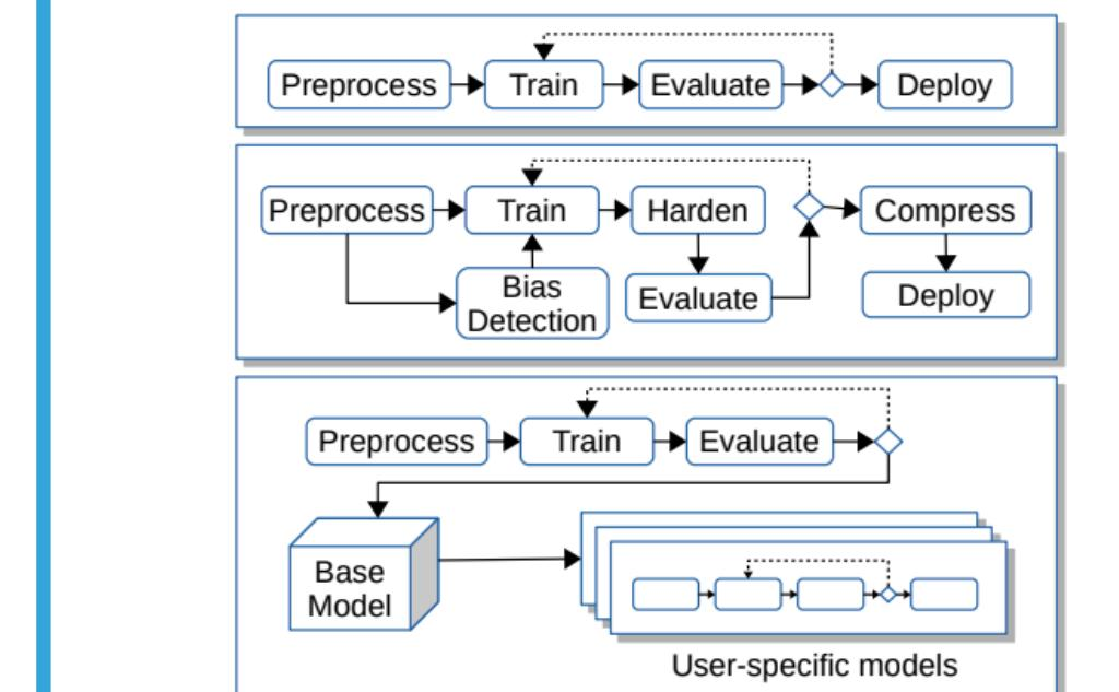
Fig. 2. Sample Pipelines: (1) Simple train/deploy pipeline, (2) complex pipeline with custom plugins enabled, (3) transfer learning pipeline with user-specific models
