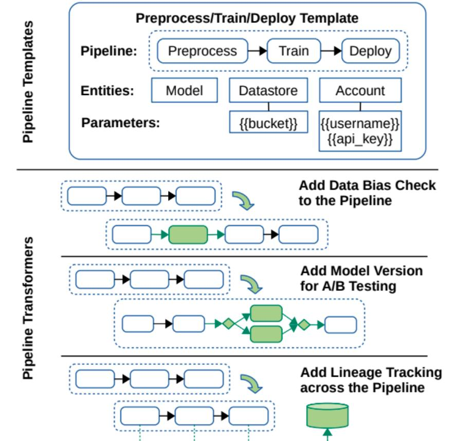
Fig. 6. Parameterizable Pipeline Templates and Transformers
